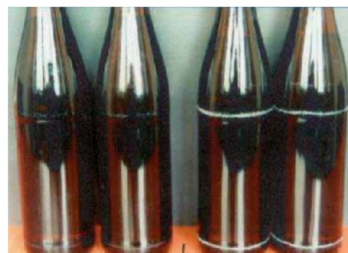
Bottles after 25 refills with and without Kercoat®
